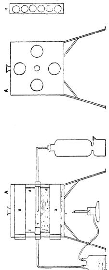
A is a copper box each side of which measures 9 inches. Four tubes a, a, a, a, run through it from front to back,  $2\frac{1}{4}$  inches diameter. In front they are open and fitted with corks. Behind they are closed. They serve to hold the asbestos drying tubes, which stand in holes in a strip of copper p, which can be pushed into the tubes a.
